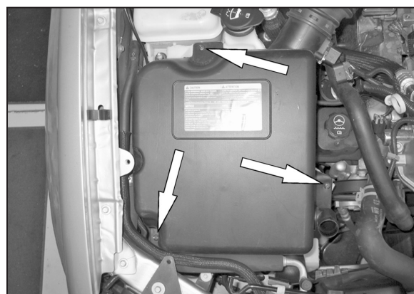
4. Loosen the three screws which secure the upper air box.
