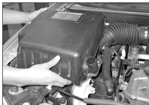
5. Remove the upper air box cover as shown.
