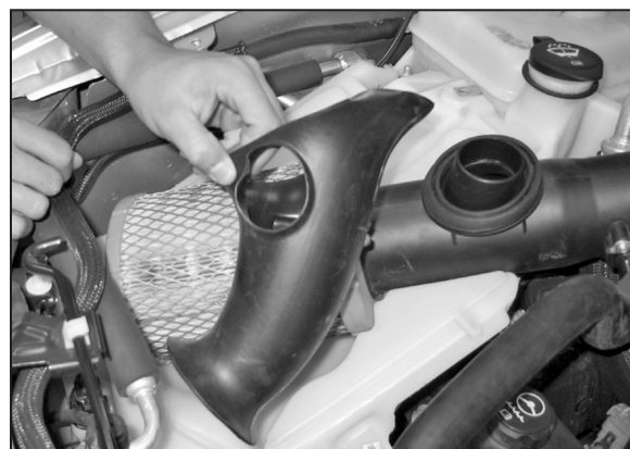
6. Remove the fresh air supply duct.
