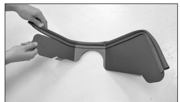
9. Install the provided edge trim onto the heat shield as shown.
