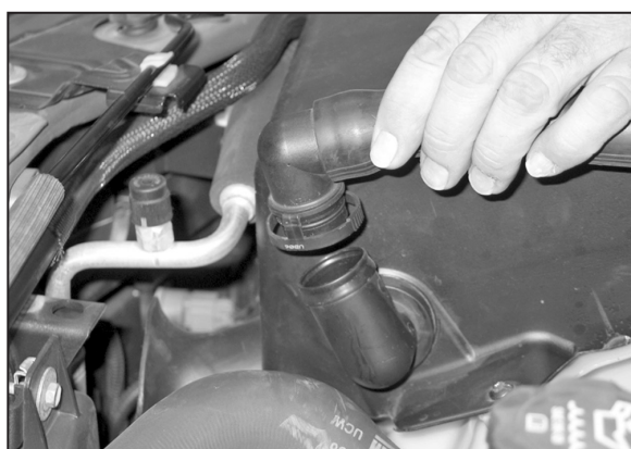
3. Depress the locking tabs and disconnect the air injection hose.
